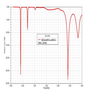
Figure 2: Simulated return loss for the MICS and ISM hand
