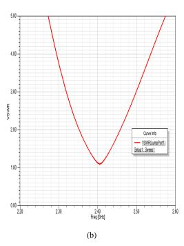
Figure 4: Simulated VSWR at: (a) MICS band; (b) ISM band
