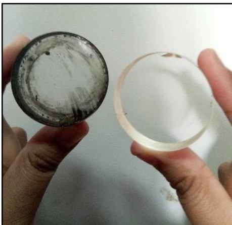
Figure 12: Comparison of Clean and Dirty Sight Glass
