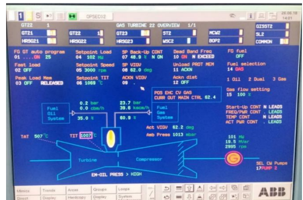
Figure 4: HMI Display in Gas Turbine
