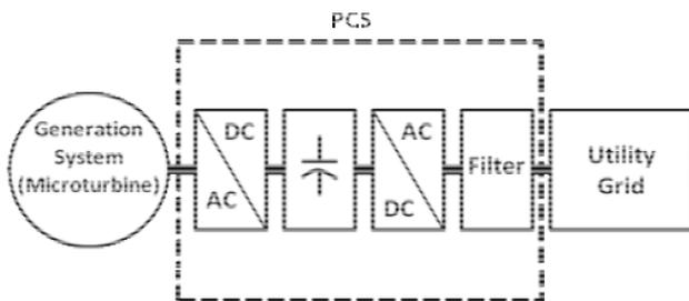
Figure 1: Microturbine Generation System
