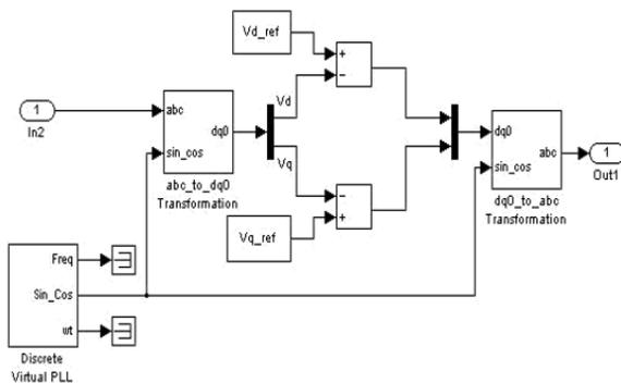
Figure 9: Isolated Mode Control System
