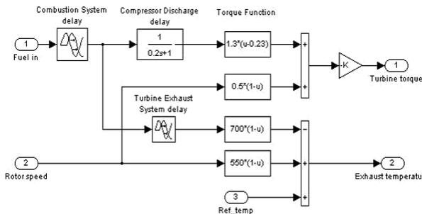
Figure 7: Compressor-Turbine System
