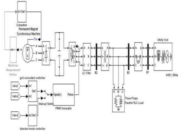
Figure 10 Simulation Model of the Microturbine Generation System
