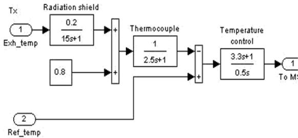
Figure 5: Temperature Control System
