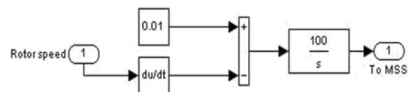
Figure 4: Acceleration Controller
