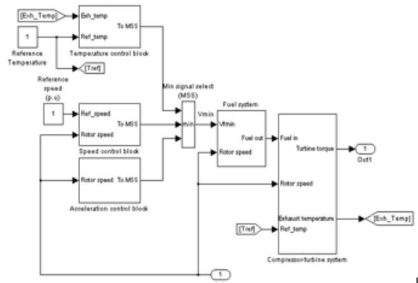
Figure 2: Model of Microturbine System
