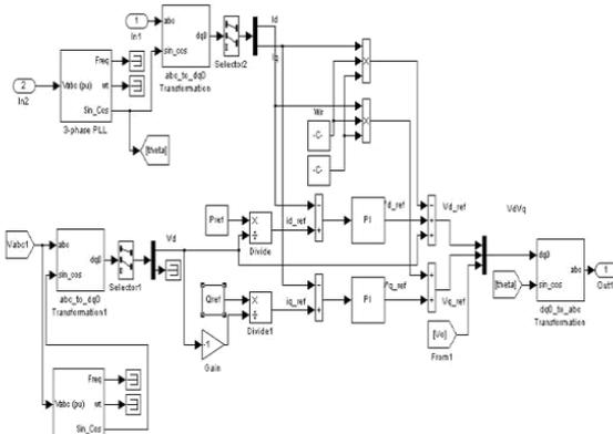
Figure 8: Grid-Connected Mode Control System
