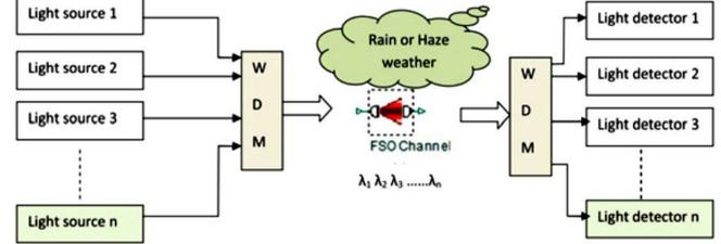
Figure 1: WDM for fiber less optical communication block diagram.
