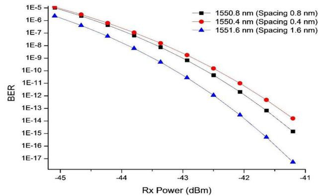
**Figure 3:** The received power for WDM with different channel spacing.
