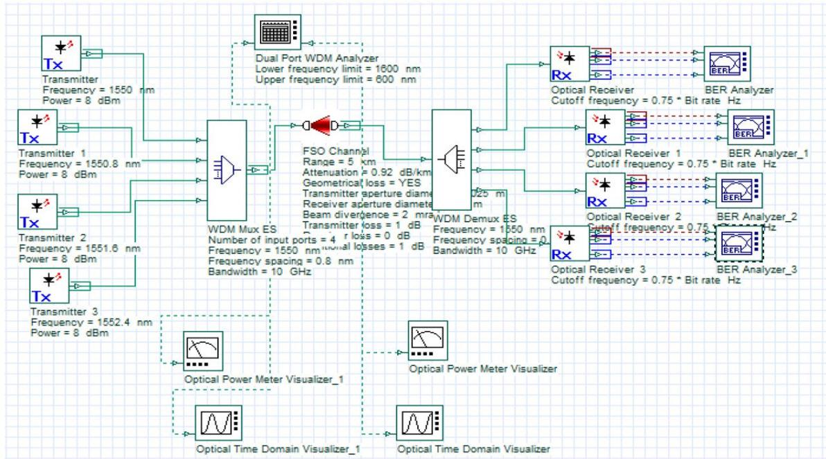
Figure 2: System Simulation Layout in Optisystem Software.
