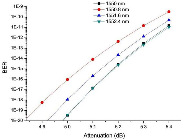
Figure 4: Variation of attenuation with BER for the four wavelengths.
