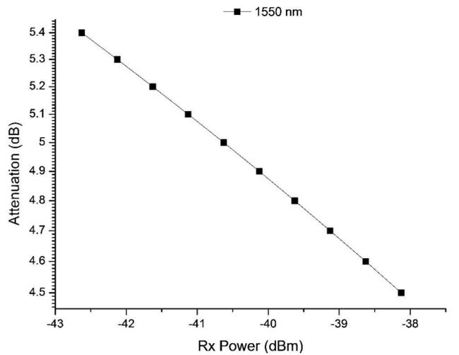
Figure 7: Optimum optical received power with the variation of attenuation.
