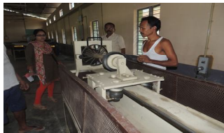
Fig 1: Cutting of bamboo culms into splints
