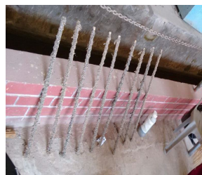
Fig 5: Bitumen coated and sand sprinkled bamboo bars
