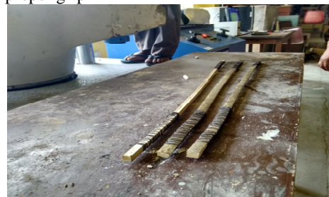
Fig 11: Bamboo ends wrapped in wire for tension test
