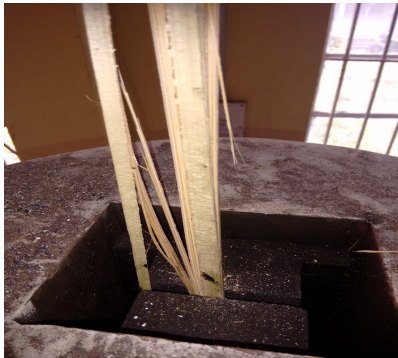
Fig 13: Failure pattern after releasing from groove.
