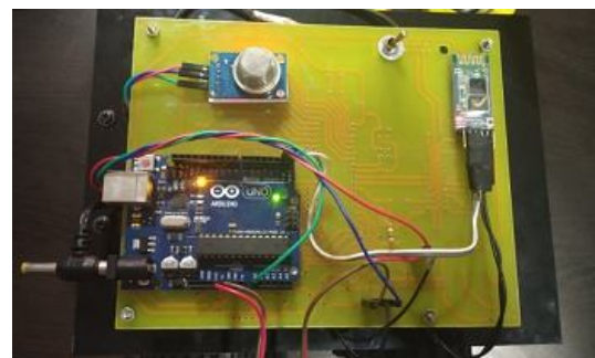
Figure 2: Top view of Gas Leakage Detector System
