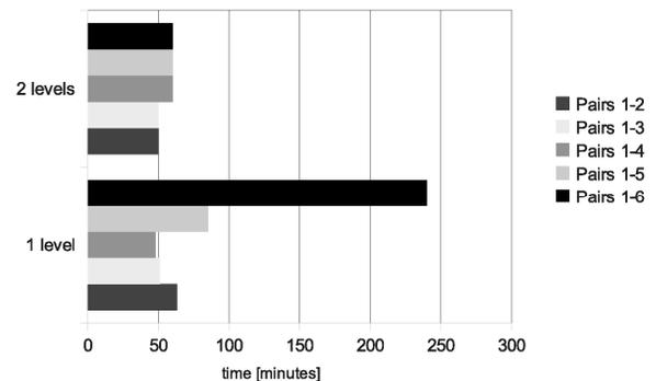
**Figure 8:** Optimization time, with multi-resolution approach (2 levels) and without it (1 level), Intel R Core™ i7, 3.2 GHz computer; all image pairs registered in parallel
