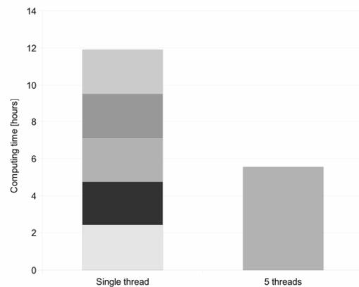
**Figure 7:** Computation time of five registration subtasks performed sequentially in a single thread or in parallel, using multiple threads on a quad-core processor (Intel™ Core® i5 M520, 2.4 GHz) computer
