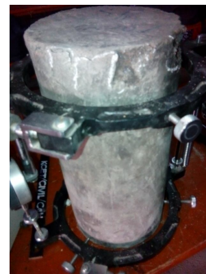
Figure 12: Cracking Pattern of Concrete Cylinder
