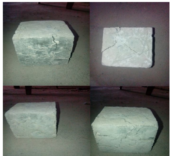
Figure 3 : Crack Patten of the concrete cube
