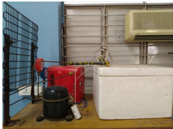
Figure 2: Cascade refrigeration setup
