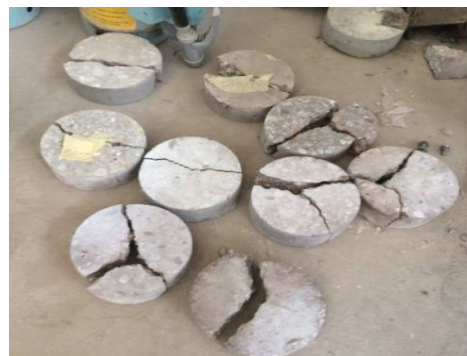
Figure 17: HSC and NSC deformed concrete specimens after conducting impact tests
