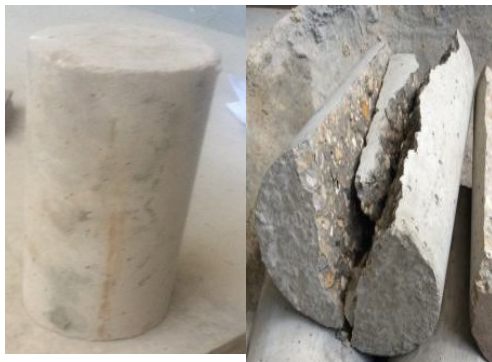
Figure 11: Concrete specimens before and after splitting tensile testing
