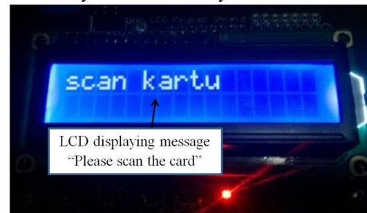
Figure 9: The System is in Active or Standby Condition if the LCD of the Controller Displays a Message "Please scan the card" (the interface uses Bahasa Indonesia ).
