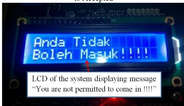
Figure 14: Message Displayed by the LCD When the Access is Denied
