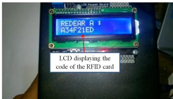
Figure 11: LCD of the Controller Box Displays RFID Code of the Card Being Scanned
