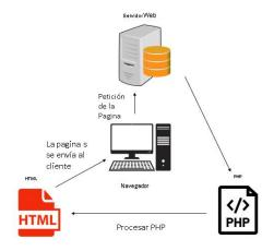
Figure 2: Client and server communication diagram
