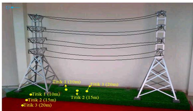
Figure 2: Data Retrieval Point of Extra High Voltage Air Duct Radiation
