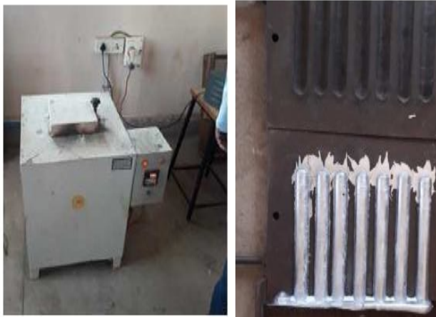
Figure 1: Equipment Used for Stir Casting and Castings Obtained in the Mould
