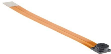
Figure 3: Camera module for PcDuino3.
