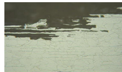
Figure. 5 : SX-6 macro and microstructure at 500x micro photo welding location corrosion area
