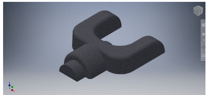
Figure 4: Making 3D CAD Cast pattern
