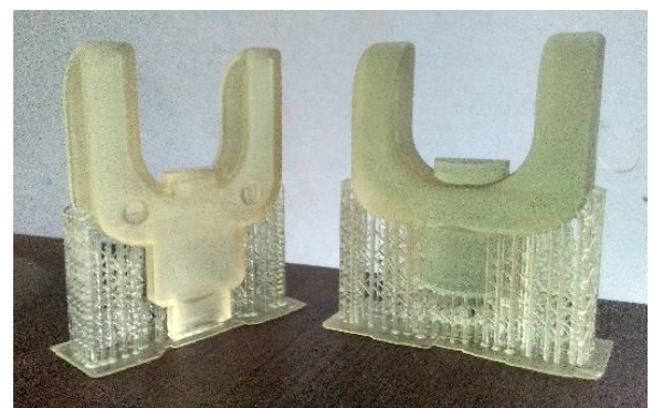
Figure 8: Results of 3D cast pattern print
