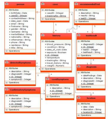
Figure 4: Low-level structure of the system using class diagrams
