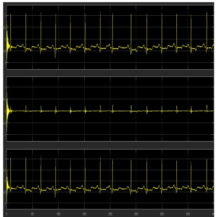
Figure 8: Simulation output of 16 - tap cascaded LMS adaptive filter structure in system generator
