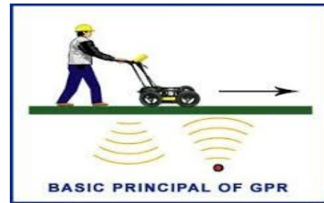
Figure 1: GPR hardware used
