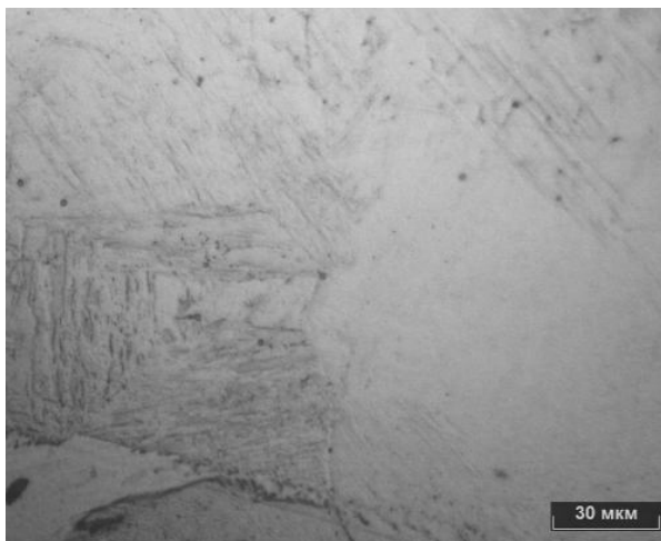
Figure 4: Microstructure view of surfacing metal of sampleNo1 at fusion boundary x 500
