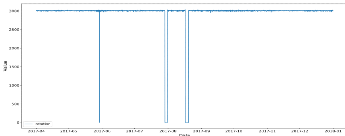
Figure 8: Turbine rotating speed signal (RPM)
