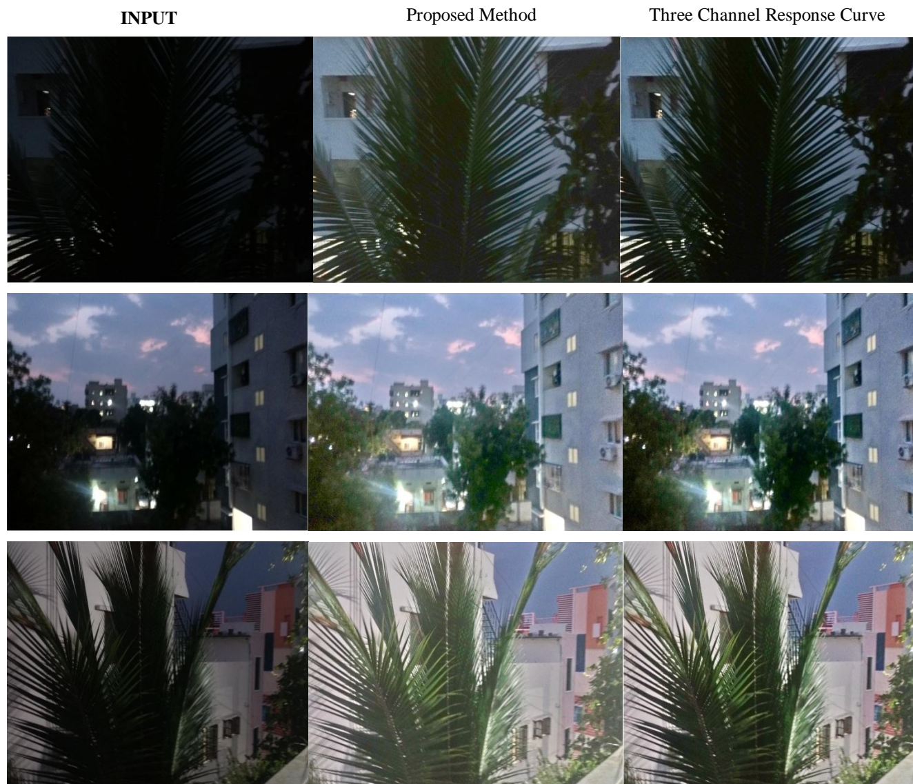
Figure 2: Screenshots from the videos before and after (using three channel curve and single approximated curve) the enhancement
