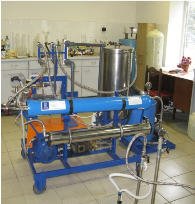
Figure 1: Two-stage reverse osmosis membrane pilot plant.
