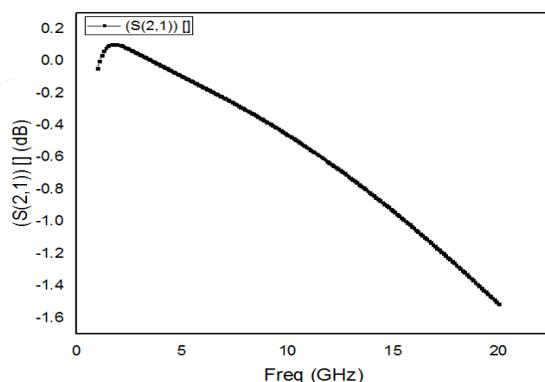
Figure 10: OFF state Insertion loss(S<sub>21</sub>).
