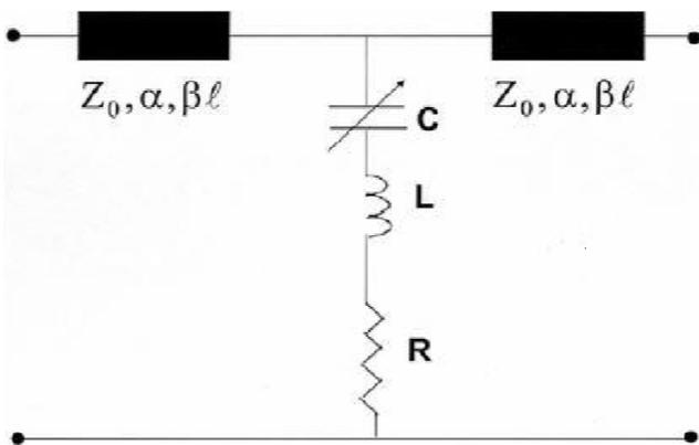
**Figure 2:** Equivalent LCR circuit for any switch.
