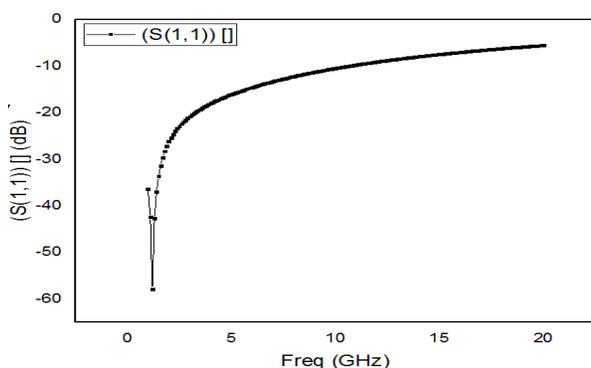
Figure 9: ON state Return loss (S<sub>11</sub>).
