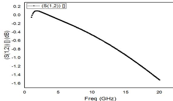
Figure 11: ON state Isolation loss(S<sub>12</sub>).
