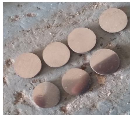
Figure 1: The samples taken from piston crown before nitriding.
