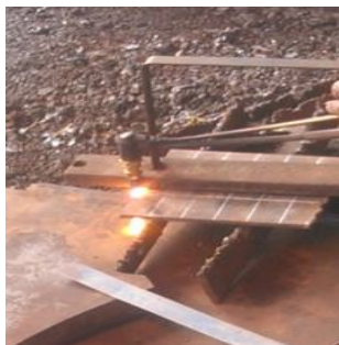
Figure 4: Samples plate for corrosion test
