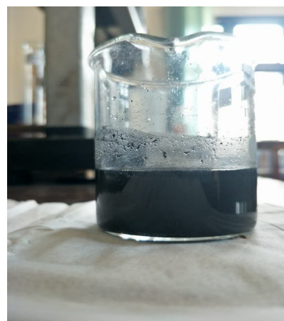
Figure 2: Solution of carbon battery rod from using batteries, H_2SO_4 and aquades
