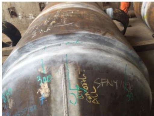
Figure 1: SFNY jacket with a lack of fusion type
