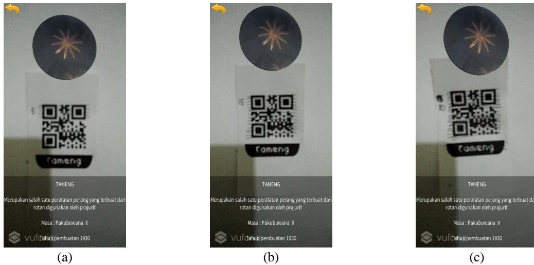
Figure 4: Test Results for Marker Condition with Streaks, (a) 5 Streaks, (b) 15 Streaks, (c) 30 Streaks
