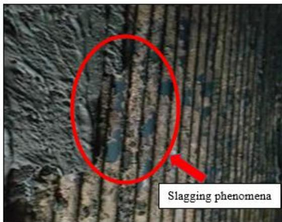
**Figure 1:** Slagging phenomena in furnace water wall
