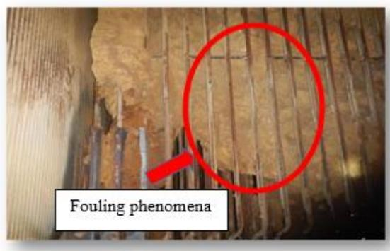
**Figure 2:** Low temperature fouling at boiler tube
