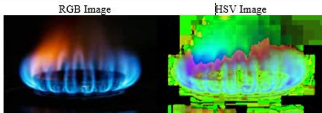
Figure 3: Converted Fluid fire to HSV Image
