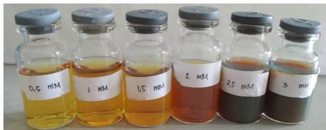
Figure 6: The color of variations in concentration of AgNPs solution at optimum conditions
