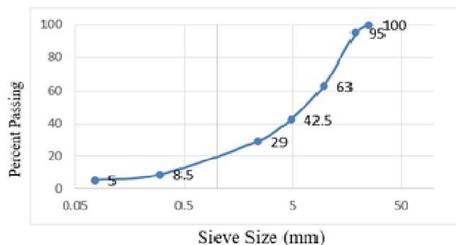
**Figure 1:** Aggregates Gradation Curve
