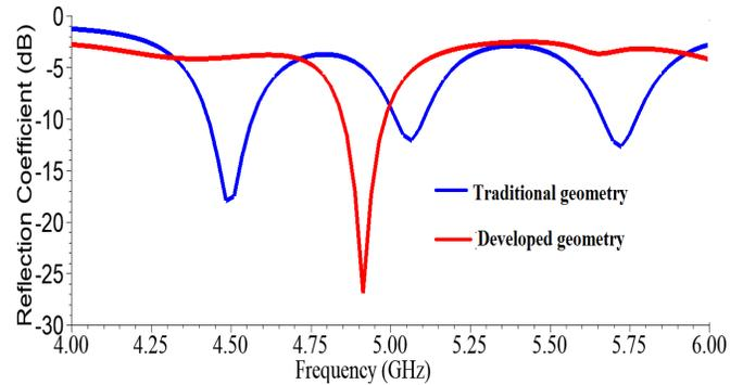
**Figure 5a:** Simulated reflection coefficient (dB) of traditional and developed antennas
