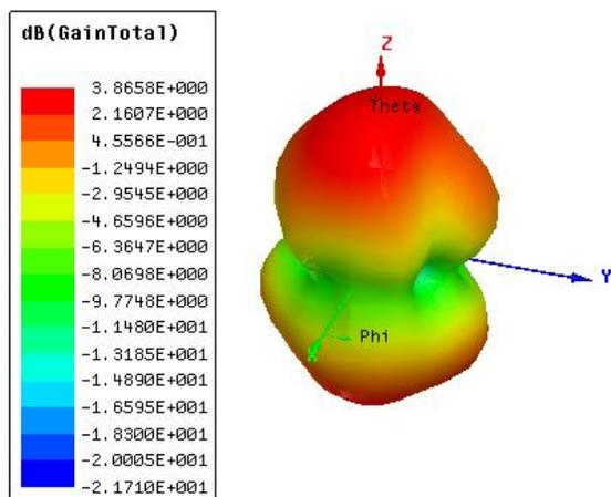
Figure 9: Simulated gain of developed antenna.
