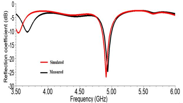
**Figure 7a:** Measured and simulated results of developed antenna
