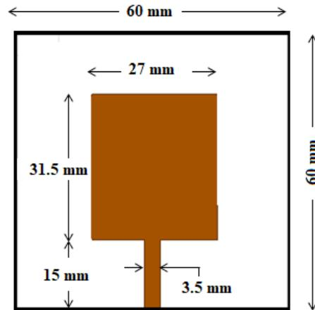
Figure 1a: Front view of traditional antenna
