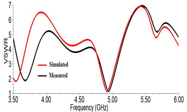
**Figure 7b:** VSWR results of developed antenna
