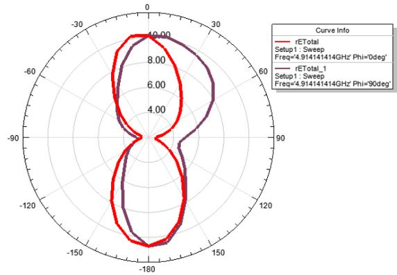
**Figure 6b:** E and H plane elevation for developed geometry
