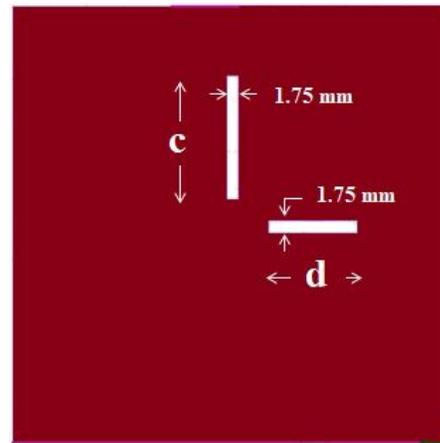
**Figure 4b:** Rear view of developed antenna with  $c=17$  mm and  $d=12.25$  mm
