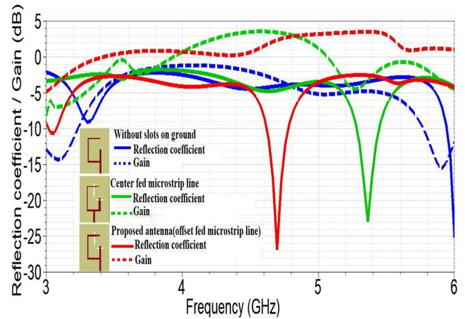
Figure 3c: Gain of antennas for change in location of microstrip line feed and introduction of slots
