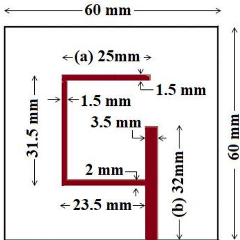
**Figure 4a:** Front view of developed antenna
