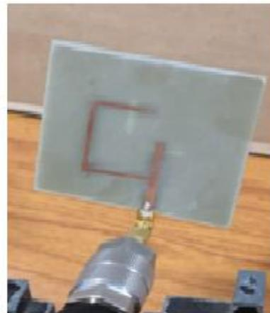
**Figure 8:** Proto type of developed geometry.
