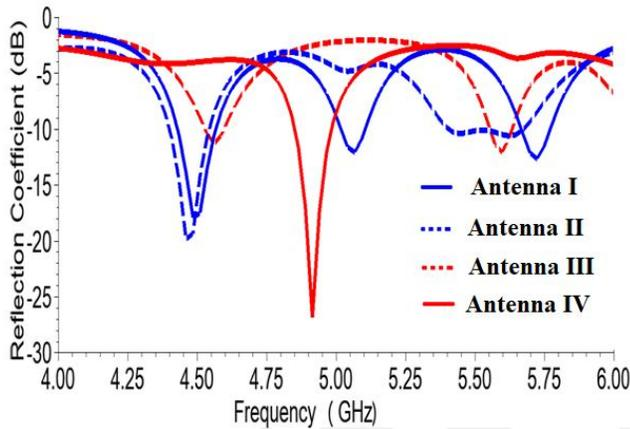
Figure 3a: Reflection coefficient vs frequency of antennas shown in Figure 2
