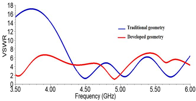
**Figure 5c:** VSWR curve of traditional and developed geometry
