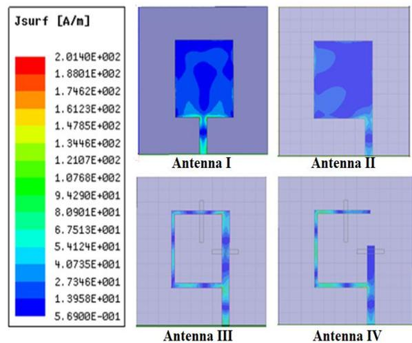
Figure 1c: Simulated current densities on patch
