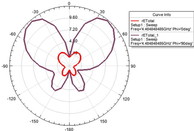
**Figure 6a:** E and H plane patterns for traditional geometry
