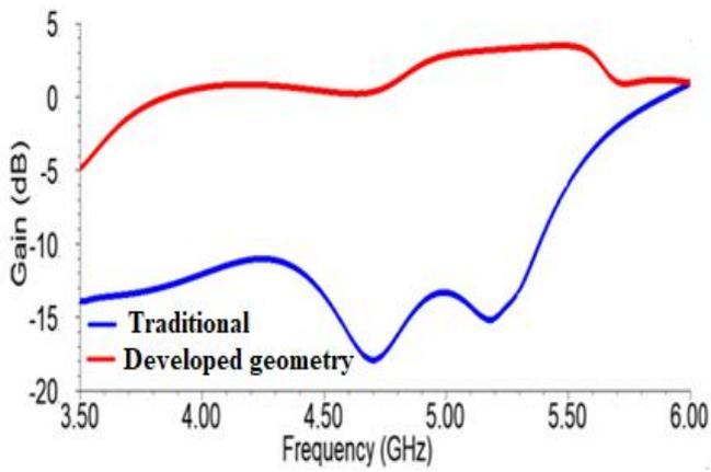
**Figure 5b:** Gain (dB) of traditional and developed geometry as a function of frequency
