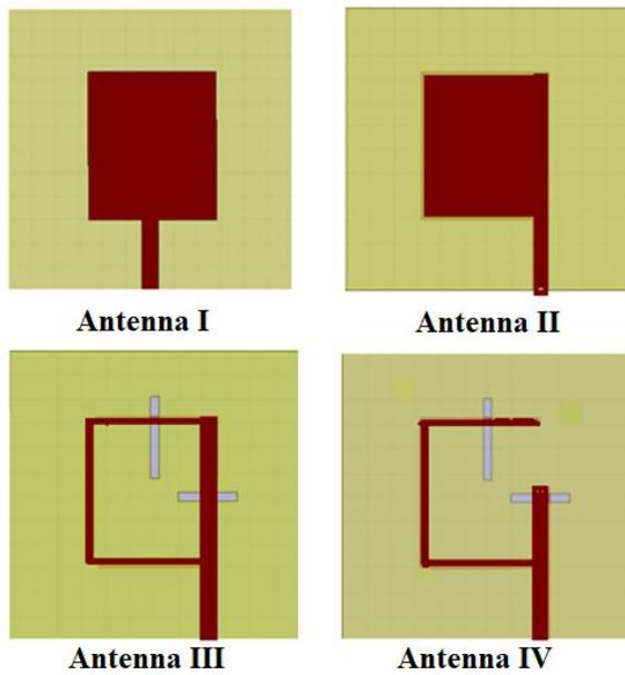
Figure 2: Design evolution of the proposed antenna
