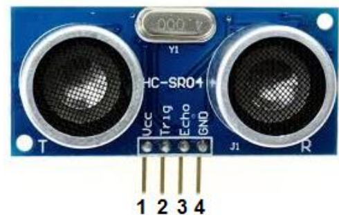
Figure 1: Pin configuration of an Ultrasonic Sensor
