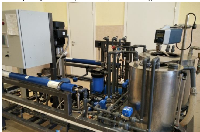
Figure 1: Two-stage reverse osmosis membrane pilot plant.
