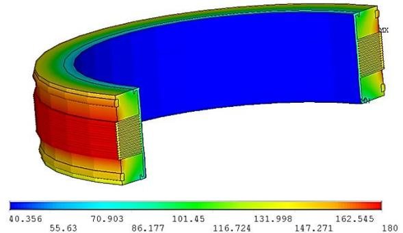
Figure 3. Temperature field distribution, °C on the surface of the TRME
