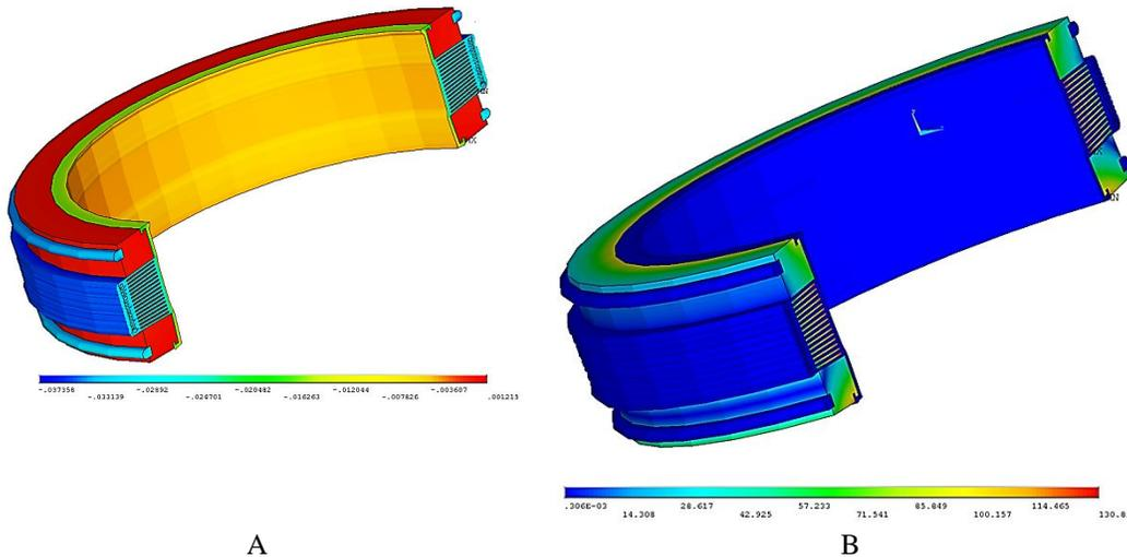
**Figure 5.** Map of the SSS parameters distribution of the thermoelastic boundary problem : A. relative axial thermal deformation of the TRME; B. intensity of equivalent stresses, MPa
