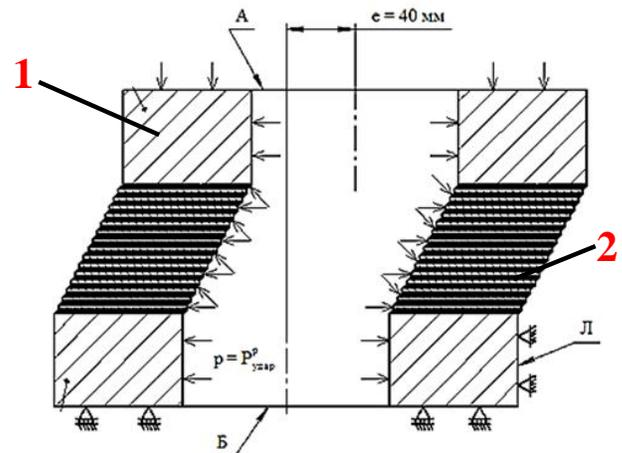
**Figure 2:** Structural design and loading scheme of the TRME with a displacement of the support rings by the value  $e$
