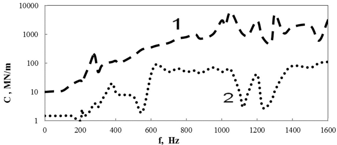
**Figure 1:** Experimentally measured vibrational transient rigidity  $C$  of sleeve-type compensators DU 80 mm (curve 1) and a compensator with TRME (curve 2) in the frequency range 0 - 1600 Hz at the water pressure of 10 MPa
