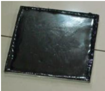
Figure 2: Graphene/E-glass fibre reinforced composite
