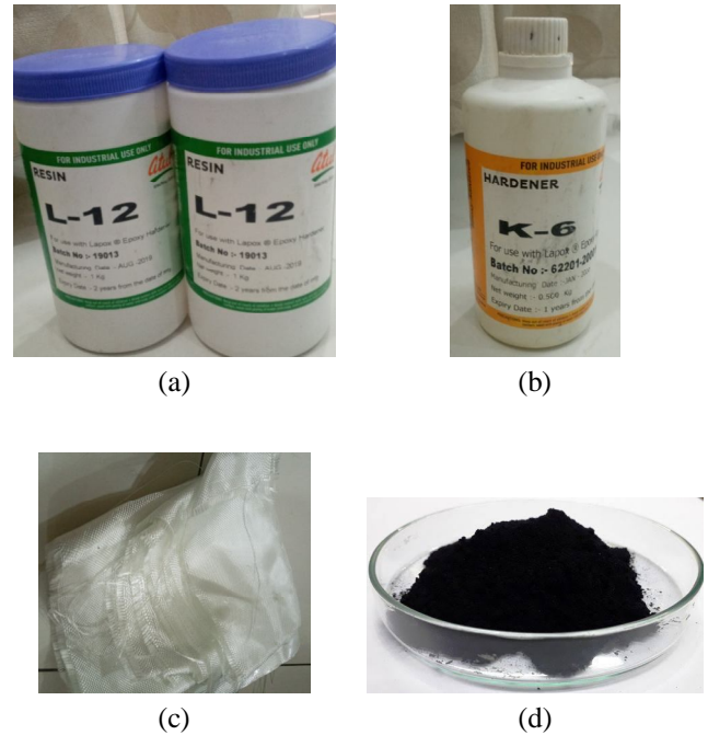
Figure 1: Material procured to prepare composite (a) Resin (b) Hardener (c) E-glass fibre (d) graphene nano particles
