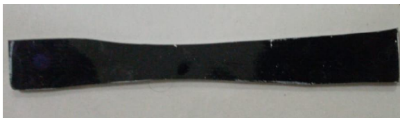
Figure 4: Dog-bone specimen of the composite
