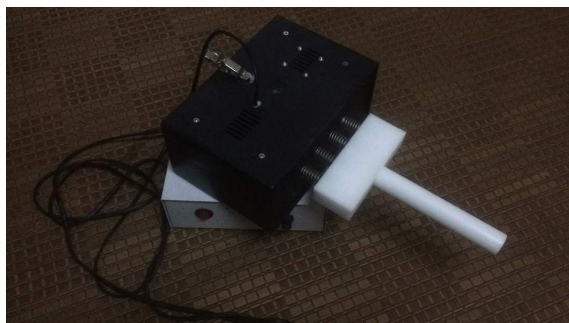
Figure 2: Handheld vibration actuator mechanism for localized vibration test
