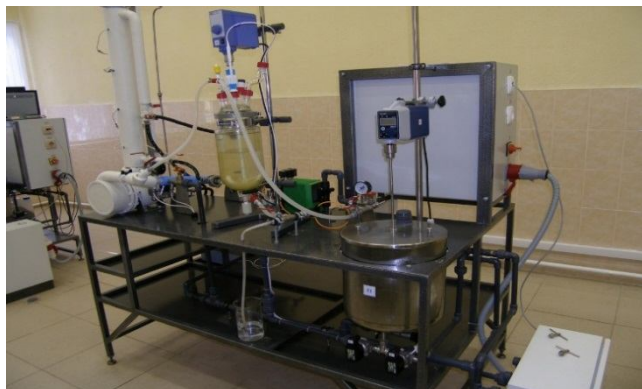
Figure 1: Experimental rotary film evaporator with hinged blades
