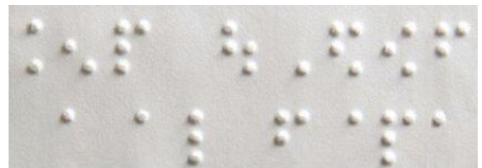
Figure 14: An example of the Braille dots embossed on paper by the printer head prototype.
