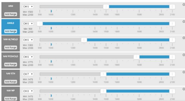
Figure 5: The setting flight modes on the control panel switches
