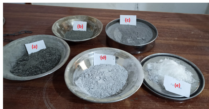
Figure 1: Materials used for production of ECC (a) sand (b) cement (c) fly ash (d) marble dust (e) PVA fibers
