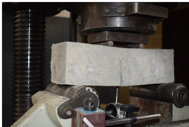
Figure 6: Experimental setup for bending test of beam specimens
