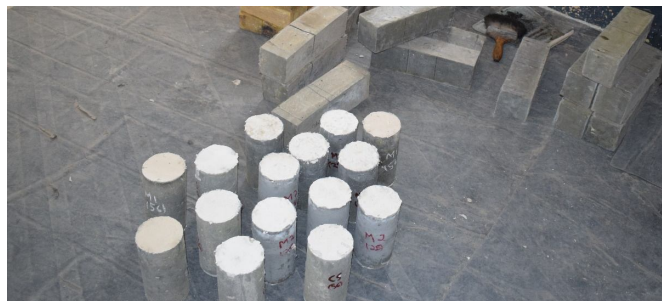
Figure 3: Gypsum capping of cylinder specimens
