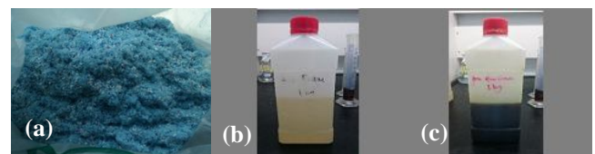
Figure 2: Raw materials (a) Grinded plastic waste, (b) Polyol, and (c) Diphenylmethanediisocyanate (MDI)
