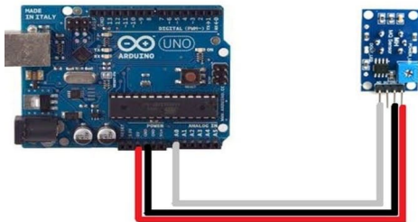
Figure-3:interfacing of arduino with mQ2 gas sensor
