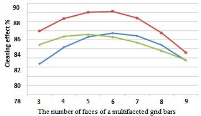
Figure 1: Graphs of changes in the cleaning effect depending on the number of faces of the grid bars
