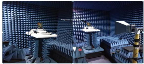
Figure 13: Testing AVA in Anechoic Chamber
