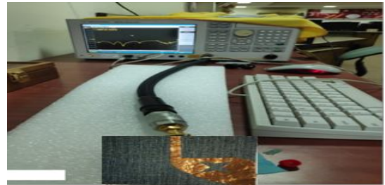
Figure 12: Testing AVA in Network Analyzer
