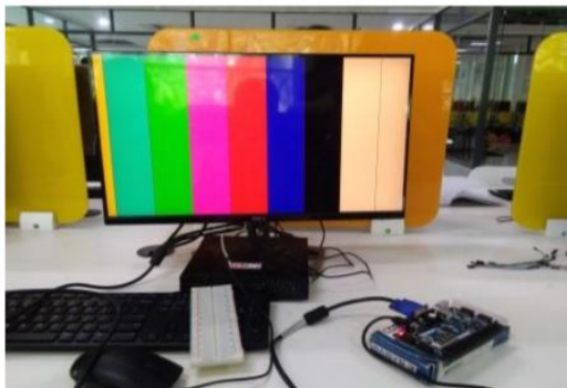
Figure 3: Basys3 FPGA Board VGA test pattern
