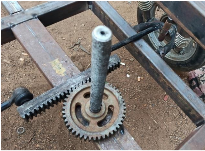
Figure 1: Spur gear & Rack setup
