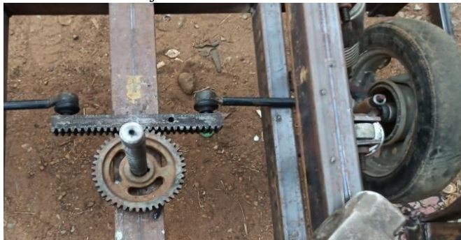
Figure 6: Spur gear connected to clamp
