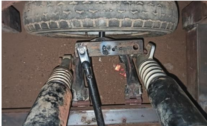
Figure 5: Shock absorber mounted on arm
