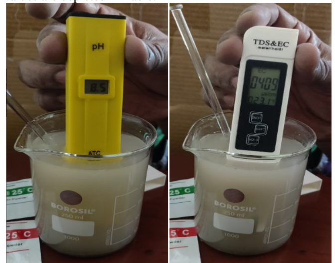
Figure 4. Measurement of the pH and EC of the Solutions
