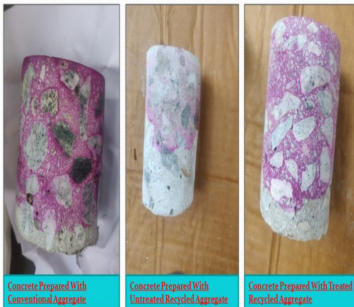
Figure 7: Effect of Carbonation on Concrete Core Sample
