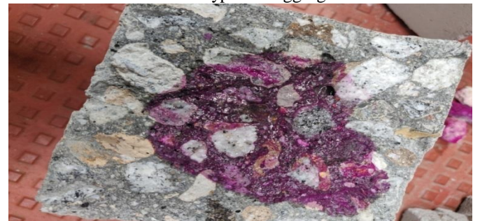
Figure 6: Carbonation effect on Concrete Mass Prepared with Different Types of Aggregates
